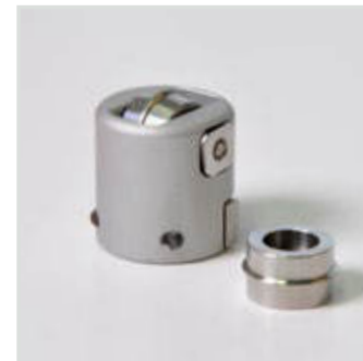
Active tangential wheel creasing tool and interchangeable wheel
